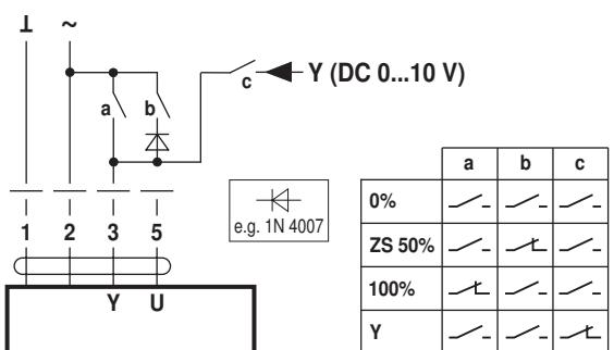
Override control with AC 24 V with rotary switch
